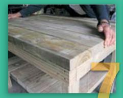
**Lay the 6 remaining pieces** on top of the frame. Line up the edges so they overhang about 250mm on each side.
