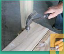
Line up shelf edges so they sit flush with the outside leg edges, then nail the seven pieces in place to secure the shelf.
