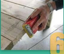
Sand the rough edges. The square edges can be slightly rounded to give a smooth finish. A sanding block is the perfect tool.
